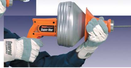
Pull Cable out of drum. Slide Shield Back to grip cable.
