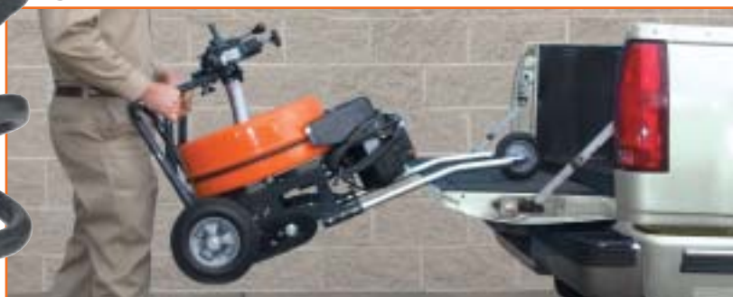
One person easily loads the Speedrooter 91 onto a truck. The swept-back handle and loading wheel give you the leverage.
