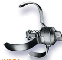
3-6HDEC Heavy Duty 3" to 6" Expansion Cutter Can pass through 3" pipe to reach and clean 6" pipe. Can be put through 4" "P" traps.
