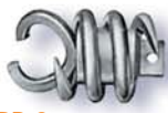
RP-2 Root Ripper Heavy spring screws into root mass, while front hook tears into stoppage. Passes through 4" "P" Traps.
