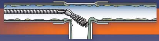
1/4" and 5/16" Down Head Lead cable down the stack – not up. For 1/4" and 5/16" cable.
